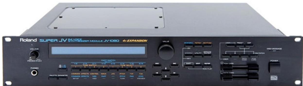
On the face of it you might think repairing or replacing the encoder would be a doddle but let me assure you, this repair is far from trivial. The very first and most important problem is that it isn't really an encoder, but a rotary pulse switch.
